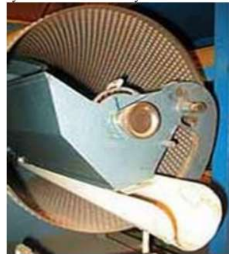
Working principle of the indented cylinder separator
