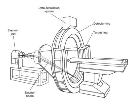
is positioned in a 47-cm scan field, to strike a curved, stationary array of detectors positioned opposite the target rings
