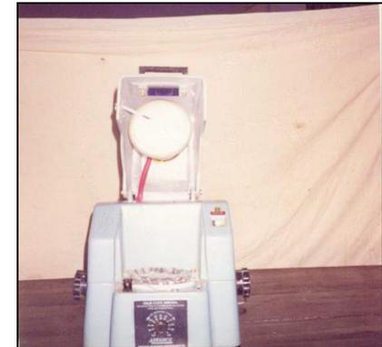
Infra red moisture balance ( top opened – showing the IR lamp)
