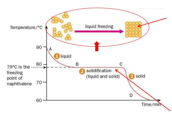
Between **B** and **C**, strong bonds are formed when particles move close together during freezing.
