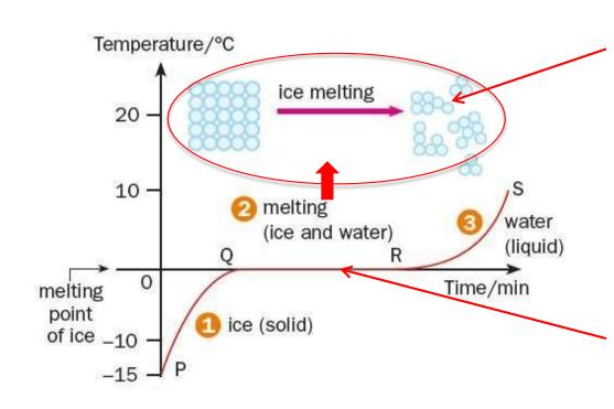
Between **Q** and **R**, thermal energy is absorbed to break the strong bonds between the particles of the solid ice.
