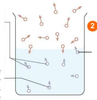
The more energetic molecules have sufficient energy to **overcome attractive forces** due to other molecules to escape from the surface into the atmosphere.
