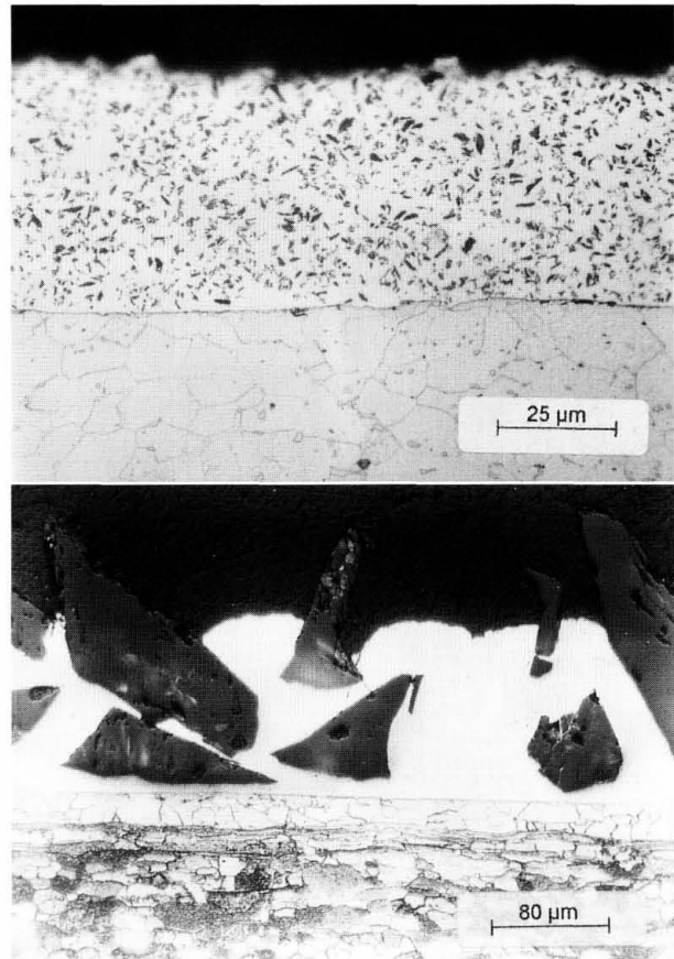
4 Cross-sectional micrographs of Ni-SiC coatings: lower coating is for grinding
