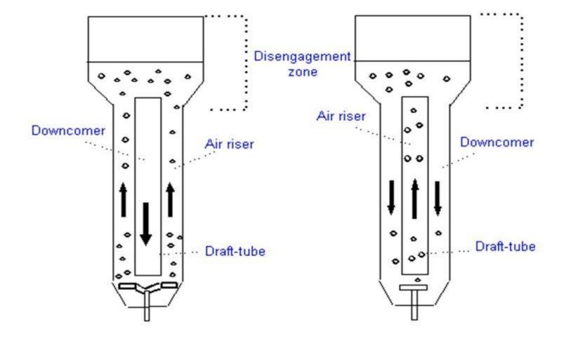
An air-lift reactor is divided into three regions by draft tube: - the airriser , down-comer , disengagement zone.
