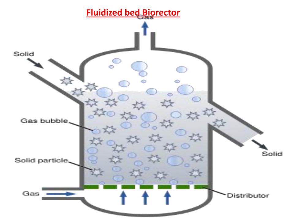
The fluidized bed reactor is has a porous plate, known as a distributor which supports the catalytic material.
