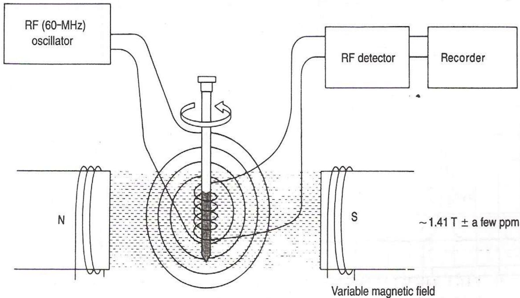
FIGURE 3.11 The basic elements of the classical nuclear magnetic resonance spectrometer.
