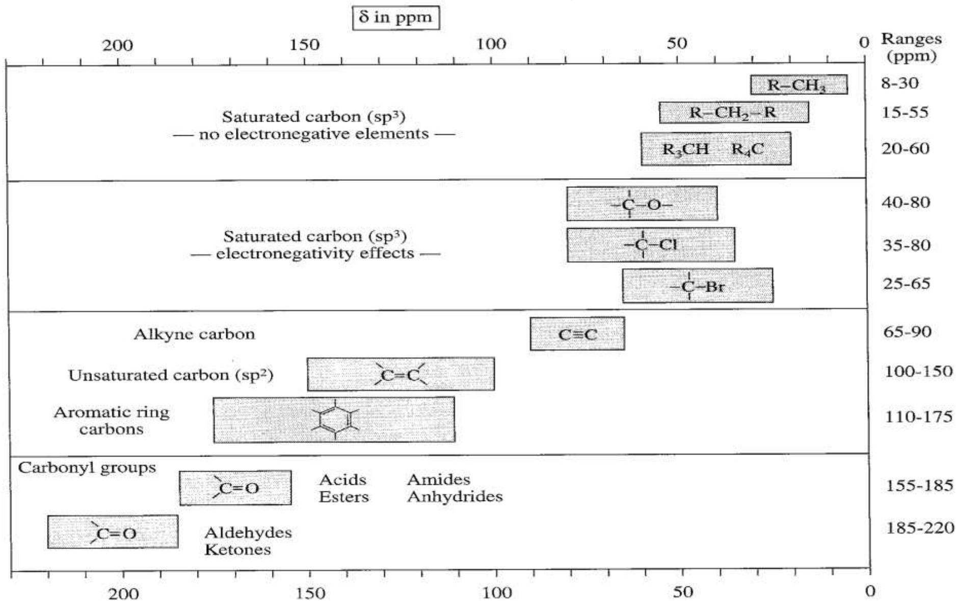
**FIGURE 4.1** A correlation chart for  $^{13}C$  chemical shifts (chemical shifts are listed in parts per million from TMS).
