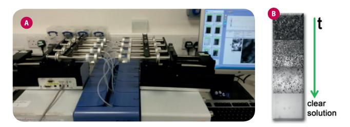
**Figure 4:** (a) Solvent addition using the Crystalline with 8 syringes attached. Each syringe can contain a different solvent composition. (b) The cameras of the Crystalline register the disappearance of the crystals as solvent is added over time.
