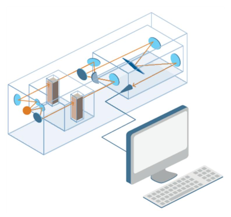
Mid-infrared is energetic enough to excite molecular vibrations to higher energy levels. The wavelength of infrared absorption bands are characteristic of specific types of chemical bonds, and infrared spectroscopy finds its greatest utility for identification of organic and organometallic molecules.
