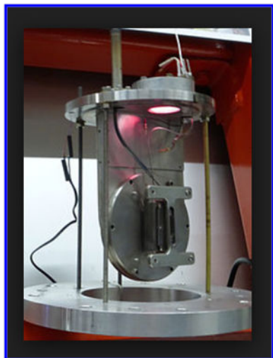
Figure 7: Plasma desorption source (by 35 years of H-ions at Fermi lab)
