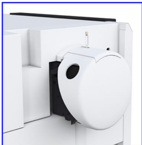
Figure 5: Electrospray Ionization source (by Agilent US).
