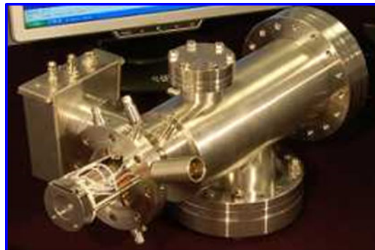
Figure 1: Electron Impact source by Kore Technology Ltd UK.
