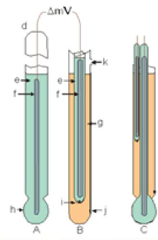
A - pH sensor B - reference half cell C - combination pH electrode (A+B) D- seal E- internal filling solution F- internal reference electrode G- external filling solution H- pH sensitive glass membrane I- internal liquid junction J- external liquid junction K- fill hole
