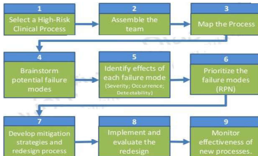
Figure 3: Hanh Phuc International Hospital adopted 9 process to conduct FMEA on Medical Gas Risk Assessment
