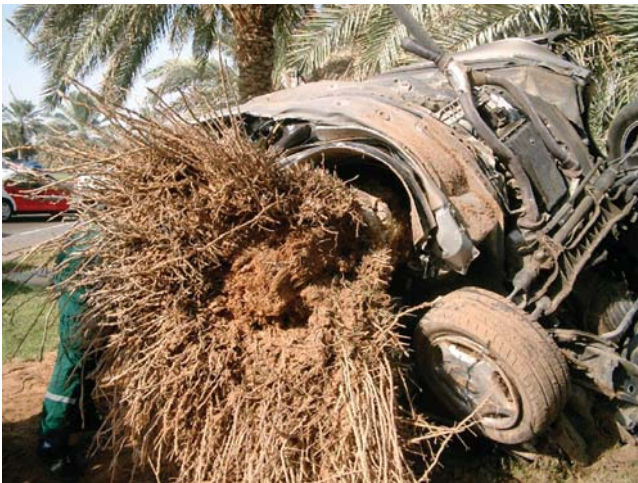
Fig. 10 Photograph shows a rollover and roof impact accident of a four-wheel vehicle. The driver was travelling at 160 km/hour and lost control of the vehicle. The car rolled over and the roof of the car impacted with a palm tree, which was pulled out from its roots from the collision.
