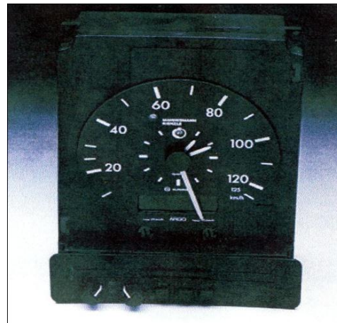
Fig. 2 and 3 illustrate two modern instruments indicating a clock speed and an odometer, a clock and buttons along with the driver and his colleague can register mode. (Most appliances recorded two diagrams where vehicle is driven by a team of two persons).
