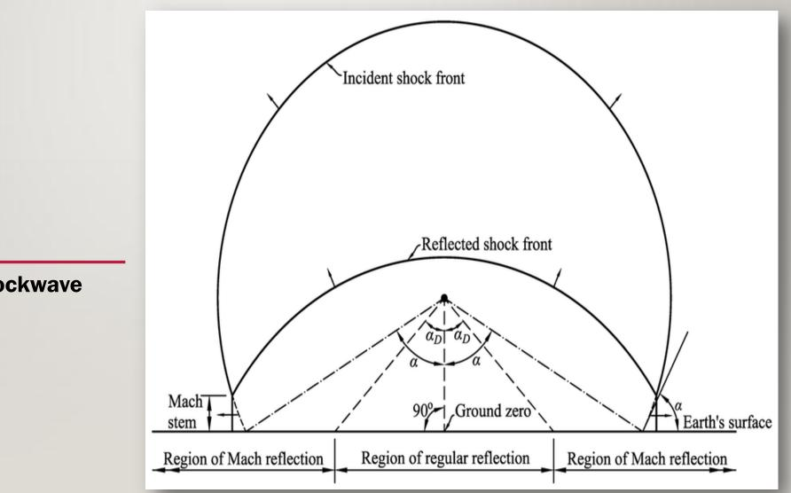
**Diagram of a shockwave**
