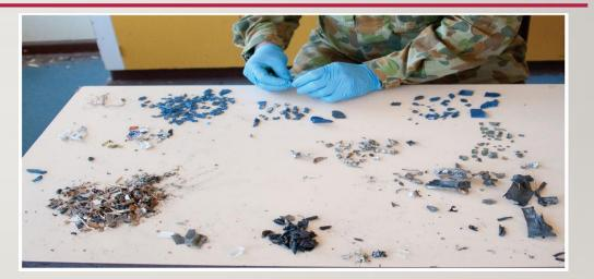
Once finished with the debris assessment, it may be possible to "reassemble" the IED into its essential components for an understanding of how the device operated.
