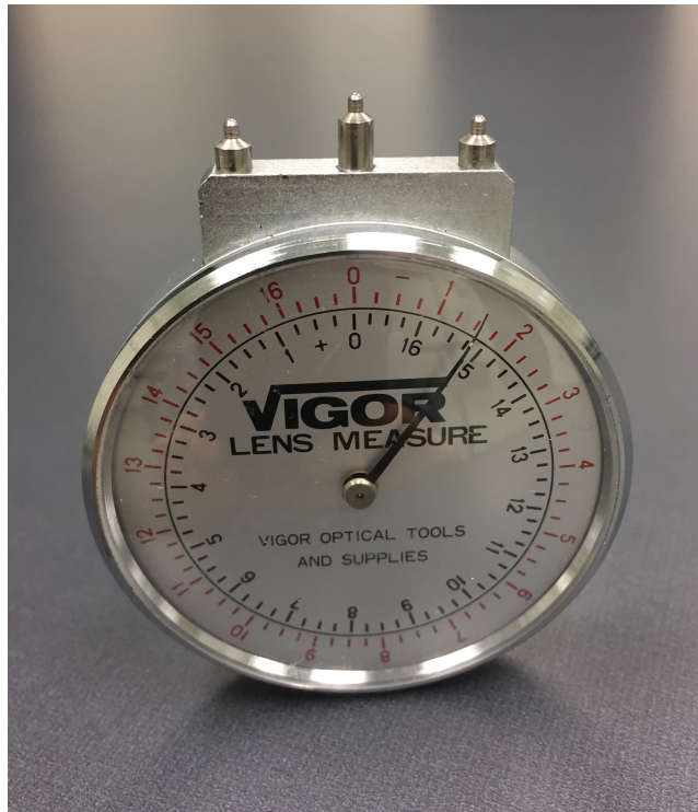
Figure 11-9. Photograph of a lens clock. The top portion with the three pins is placed against the lens surface. Since the center pin is movable, it can measure the surface's sagittal depth, which is converted to the base curve displayed on the dial. The base curve is the surface's power assuming the lens material has an index of 1.53.
