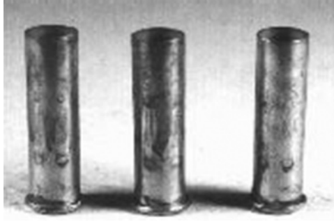
Figure 4.22 Perforated chamber marks on fired cartridge case.
