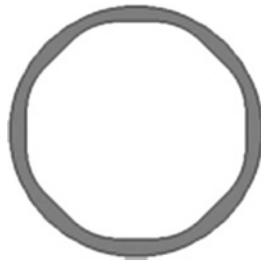
Figure 4.10 Conventional eight-groove rifling.
