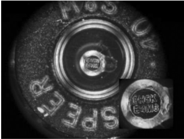
Figure 8.3 Firing pin impression with laser-etched serial number.
