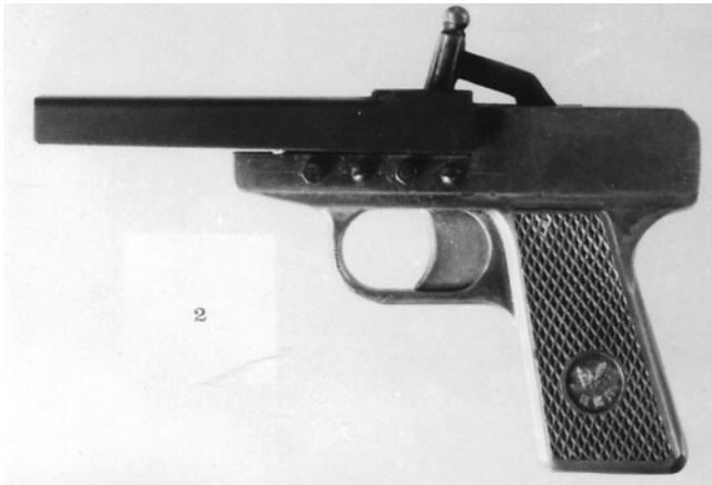
Figure 5.13 Converted, 0.22" calibre, muzzle-loading blank pistol.
