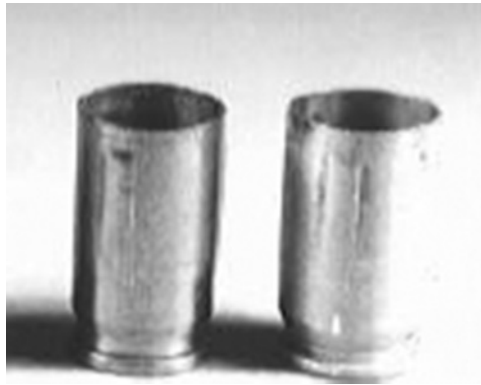
Figure 4.20 Scoop chamber marks on fired cartridge case.
