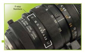
of light (more light= brighter image) to pass through the lens. Higher f-stop numbers indicate that smaller amounts of light (less light = darker image) can pass through. The appropriate f-stop setting varies per situation, based on the lighting in the environment and the brightness of the object(s) in the shot.
