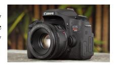
through the lens and see exactly what will be captured. When the shutter button is pressed on a mechanical SLR, the mirror flips out of the light path, allowing light to pass through to the light receptor and the image to be captured.
