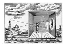
Camera Obscura is the natural optical phenomenon that occurs when an image of a scene at the other side of a screen (or for instance a wall) is projected through a small hole in that screen as a reversed and inverted image (left to right and upside down) on a surface opposite to the opening. The surroundings of the
