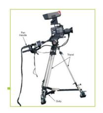
**Pan handle:** A device attached to the back of the tripod head that allows the camera operator to move the tripod head while standing behind the tripod.
