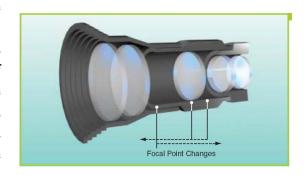
**Variable focal length lens:** A lens in which the optical center can vary its position within the lens assembly, varying the focal length measurement as well. Also called a zoom lens.
