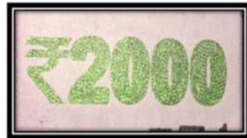
Figure 8A: Optically variable ink (green)
