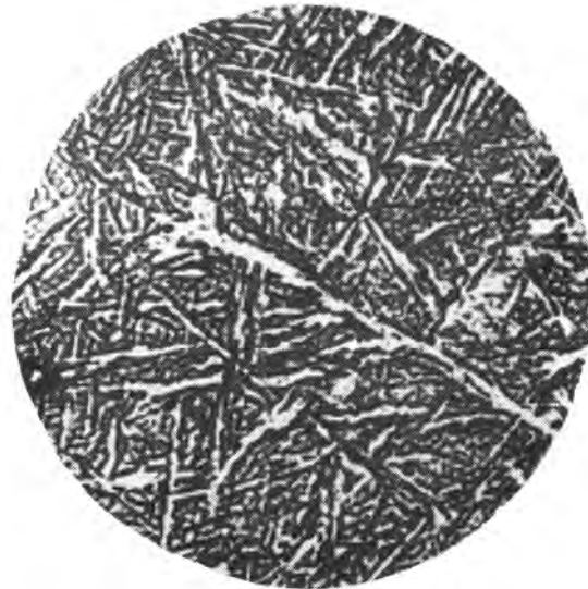
Figure 5.6 Microstructure showing coarse accicular martensite ( \times 300 ).
