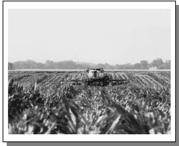
Figure 18.2 Using a mechanical detasseler to emasculate corn. (Courtesy of Pioneer Hi-Bred Seed Company.)
