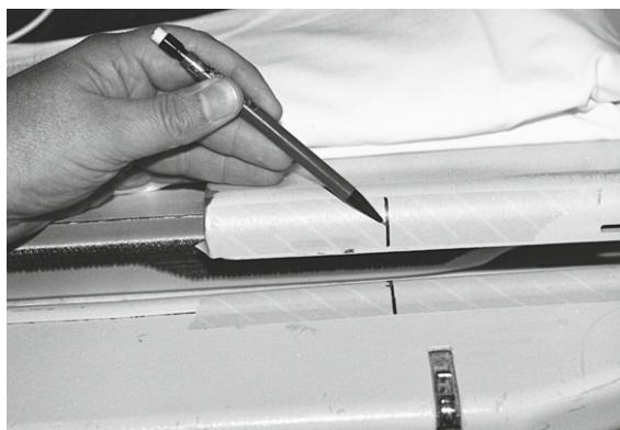
FIGURE 20-15 Two strips of tape on the bed to determine bed backlash for both the moveable and stationary parts of the bed. The two pencil marks opposite each other define the starting or zero location of the bed.
