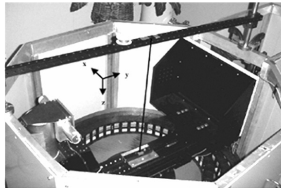
FIGURE 13-17 An inside view of the flat-panel CsI amorphous silicon TFT digital radiography detector used in the FD-CT scanner for imaging the breast. (From Kwan ALC et al: Evaluation of the spatial resolution characteristics of a cone-beam breast CT scanner, Med Phys 34:275-281, 2007. Reproduced by permission of the American Association of Physicists in Medicine.)
