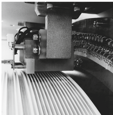
FIGURE 5-13 Slip ring based on the cylindrical design characteristic of the Picker PQ-2000 CT scanner. The brushes glide in contact grooves on the stationary slip ring. (Courtesy Picker International, Cleveland, Ohio.)
