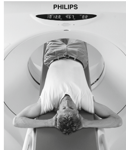
FIGURE 7-5 The gantry aperture is the opening in the gantry in which the patient is positioned for the examination. The diameter of the aperture shown is 700 mm. (Courtesy Philips Medical Systems.)
