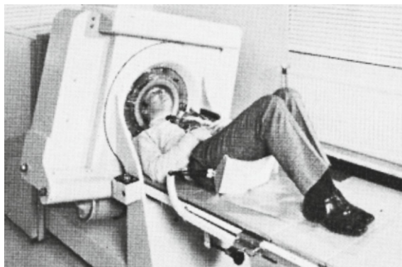
FIGURE 1-2 First-generation model of a CT head scanner. (Courtesy Thorn EMI, London, United Kingdom.)
