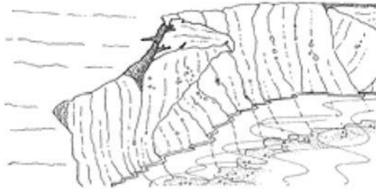
Fig. 12.2. Undercutting of the bank toe, a sign of bank scour.
