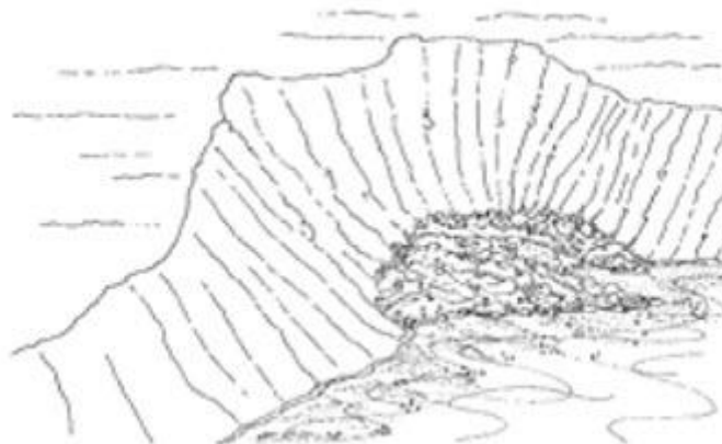
Fig. 12.3. Slumping is a Common Type of Mass Failure.
