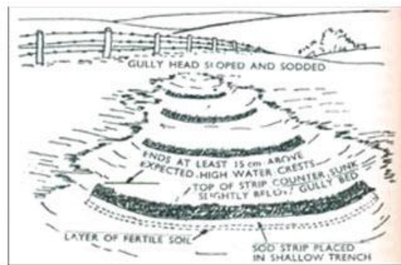
Fig. 7.4B. A series of sod-strip checks in a small gully. (Source: Agr. Handbook No. 61. USDA, SCS).
