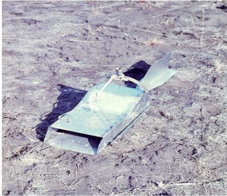
Fig. 20.1. A Commonly Used Type of Bed-load Sampler.
