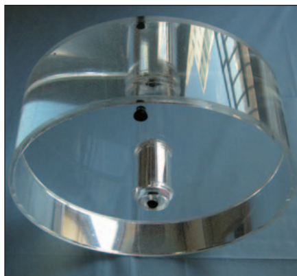
Fig. 1 —Photograph shows 300-mm-diameter cylindrical water phantom used to mimic abdomen of intermediate-size patients. For imaging, 25-mm-diameter tube filled with diluted contrast material was inserted into center of phantom.
